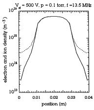
Fig. 1 Steady-state, time-averaged electron (——) and  $N_2^{\star}$  ion (---) density.
