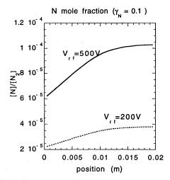
Fig. 8 Mole fraction of the N atoms calculated for different values of  $V_{\rm rf}$  and for  $\gamma N = 0.1$ .
