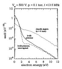
Fig. 4 Steady-state, time-averaged electron energy distribution function.
