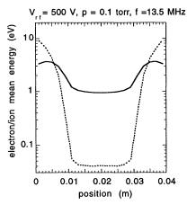
Fig. 2 Steady-state, time-averaged electron (——) and  $N_2^+$  ion (---) mean energy.
