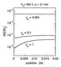
Fig. 7 Mole fraction of the N atoms calculated for different values of  $\gamma N$ .
